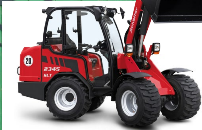
The SLT machines of the 23 series are also available with a cab, and still with a machine height of only 1.95 m (depending on tyres).
