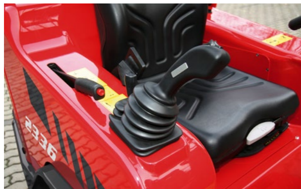
The slightly twisted joystick position simplifies operation.
