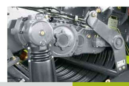
Maintenance-free for peace of mind. High-quality overload clutches immersed in an oil bath conveniently protect the QUADRANT against overload.
