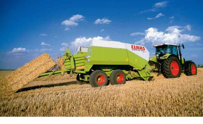
With the 83 in (2.1 m) wide CLAAS premium pick-up and the POWER FEEDING SYSTEM, the QUADRANT is perfectly equipped to gather up even the widest swaths at a high working speed.
