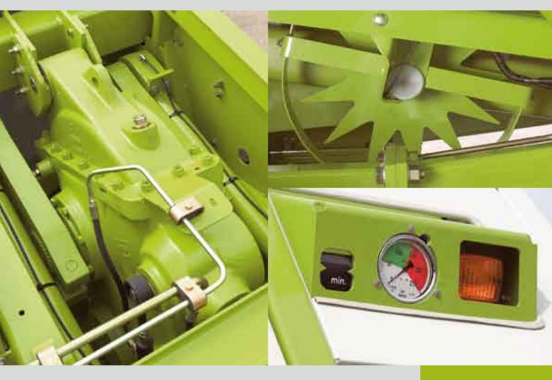
Clearly visible pressure gauge. The large-size pressure-gauge dial informs the driver of the bale density at a glance.
