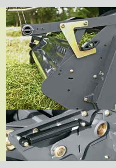
The pressure-accumulator suspension means the pick-up travels evenly over the ground. The large caster guide wheels keep you safely on track.
