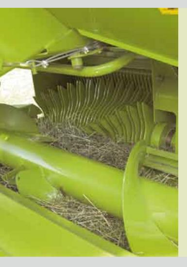
Higher input performance. On the QUADRANT 2100 ROTO CUT, a generously sized, continuous 83 in (2100 mm) wide auger merges the crop quickly and surely across the 31.5 in (800 mm) rotor chop width.
