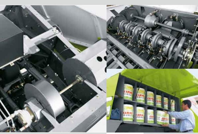
The best knotter cleaning far and wide. The TURBO FAN system cleans the knotter device with a constant airflow from two turbines.
