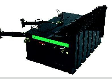
Reliable compression. CLAAS quality through and through. The heavy rollermounted ram is guided securely on the hardened tracks. Special cleaners keep the contact faces clean.
