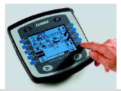
Crop moisture content indicator. The optional moisture sensor tells the driver about the quality of the crop being baled – valuable information which allows you to adjust the baling pressure accordingly.
