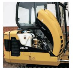
**Lift Up Side Cover.** Access to the implement valve and hydraulic tank is convenient through a lift up side cover.
