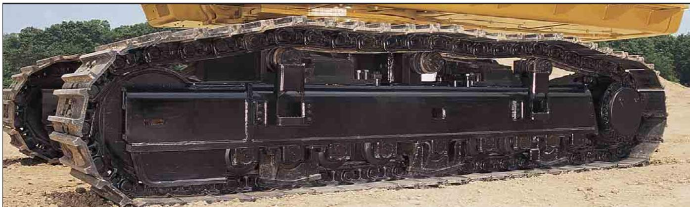
**Carbody.** To meet transportation requirements, the 385B L undercarriage is of a variable gauge type. This design allows the track roller frames to be bolted to the carbody, enabling the machine to be made narrower for ease of transport. The carbody utilizes a new columnless design which allows the swing bearing to be directly mounted on the top plate for more rigidity and strength.
