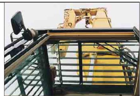
**Falling Object Guard.** An ISO 10262:1998 certified falling object guard on top and front of the cab is standard. The cross-bars of the top guard are angled in line with the operator's sight for enhanced visibility of the work tool. The front guard swings out for easier windshield cleaning.
