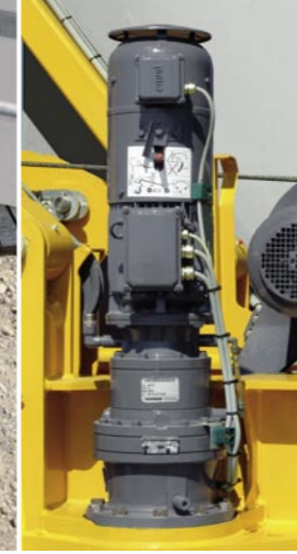
The EDC slewing gear.
