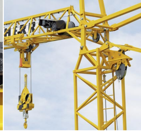
The trolley travel gear.
