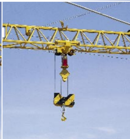
Patented automatic rope re-reeving.
