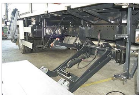
DH-RC 750 kg Side-mounted to load / unload through the side doors of the vehicle body
