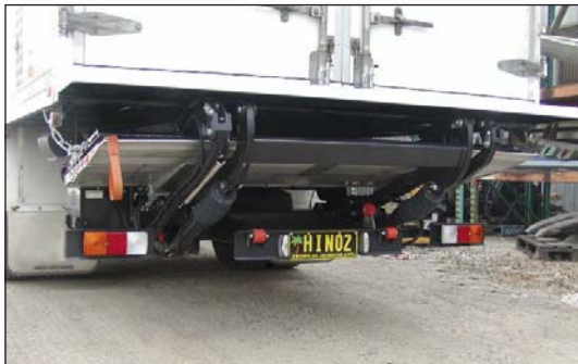
DH-RM 1500 kg - 1450 mm steel / alu platform with 3-piece fixed bumper bar
