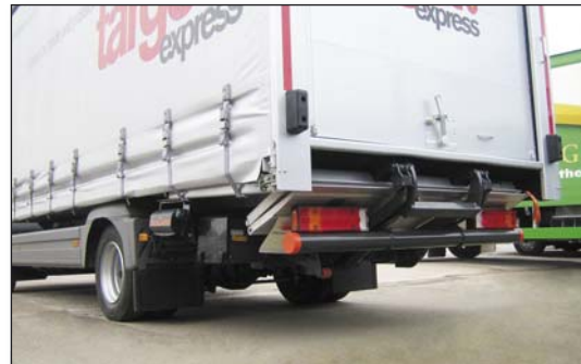
DH-RC 1000 kg - 1280 mm full alu platform with round bumper bar mounted to the lift arms
