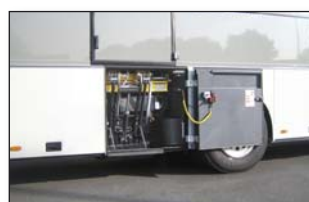
DH-RC 750 kg Side-mounted to load / unload through the side doors of the vehicle body
