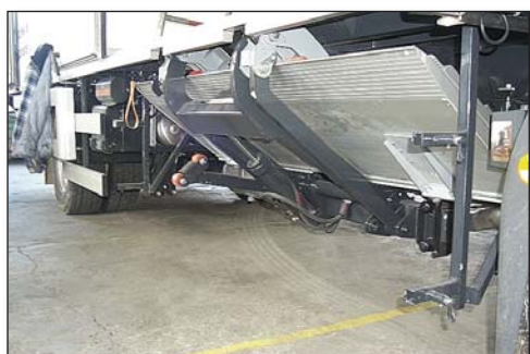
DH-RC 750 kg Side-mounted to load / unload through the side doors of the vehicle body
