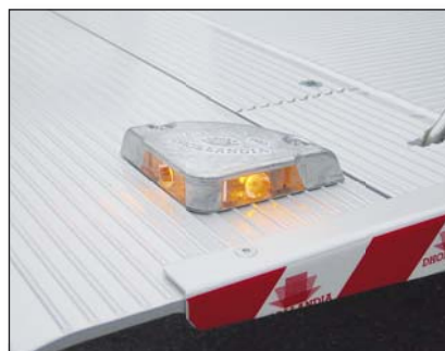
S090 Platform lights mounted onto the platform
