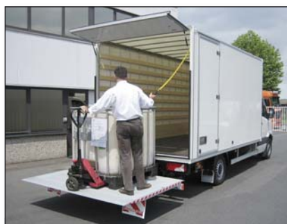
S001 2-button wander lead with spiral cable
