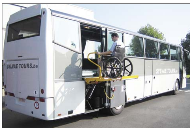
DH-RB 500 kg Tuck away lift for higher floor heights, e.g. for passenger / wheelchair handling
