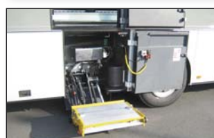
DH-RB 500 kg Tuck away lift for higher floor heights, e.g. for passenger / wheelchair handling
