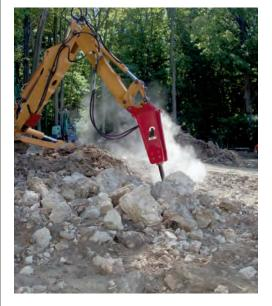
One or more of over 2,500 customized hydraulic kits from Allied provide components for mounting the Model AR 85B on backhoes and excavators. The Model AR 85B requires 13 to 27 gpm at 1,400 to 1,750 psi and it breaks at a rate of 500 to 750 blows per minute.
