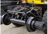
As option available: Friction Drive System available for 1404 ZW with track width 1000, 1435 and 1524 mm.
