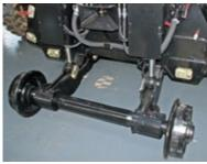
CARSY System available for 1404 / 1604 ZW with track width 1435 / 1524 and 1600 mm.
