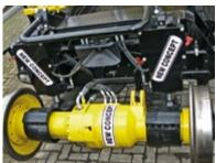
As option available: Hydrostatic Drive at 1604 ZW with track width 1000 / 1435 mm track width. Perfect setting for permanent - brake controlled high ride drive on tracks to prevent damage and excessive wear of the tyres.
