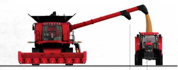
Standard unloading system at 88l/s (5130) and 113l/s (6130, 7130)
