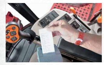
Ideal for contractors, on combines equipped with yield monitoring a job printer allows performance and area data to be printed and handed over to the customer at the end of each job.
