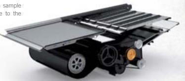
But it's not just the rotor that makes the Axial-Flow® different. The Cross Flow cleaning system which follows the separation process uses chevron-shaped fins to create a uniform vortex along its axis to generate high volumes of air throughput. Unlike conventional systems, there are no air pockets created – distribution is consistent across the underside of the sieves – and fan speed is fully adjustable to cater for finer-seeded crops.
