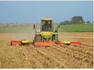
The CM conditioner for 9.0 m (29'6") working widths A flail topper is available as optional specification from our system partner Van Wamel B.V.. The unit will boost machine utilization and effectively fight the corn borer.
