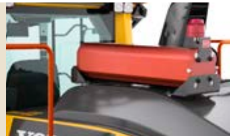
Fire suppression system
