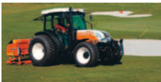
1 Precision ground hugging with axle-guided front hitch
