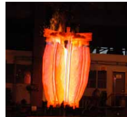
12 hours carburising heat treatment for each mouldboard
