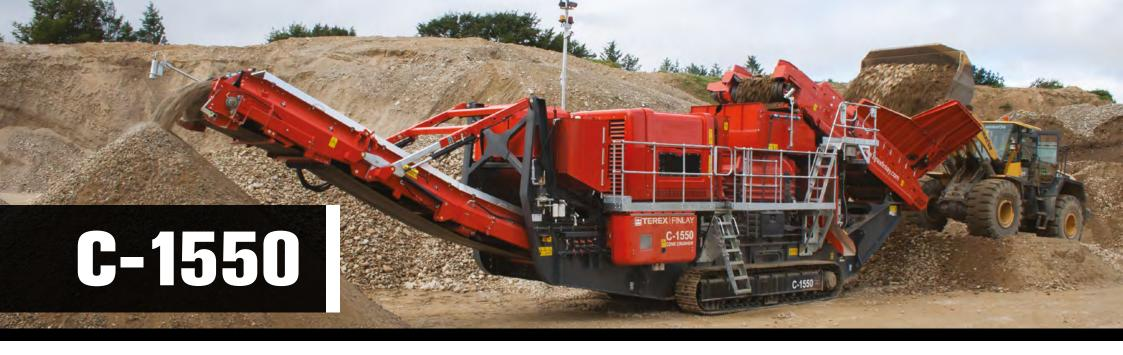
The Terex® Finlay C-1550 is a high capacity and aggressive cone crusher for the surface ore mining and aggregate industries. This efficient and productive machine incorporates the proven Terex® 1300 cone crusher with direct variable clutch drive, automatic tramp relief and hydraulic closed side setting (CSS) adjustment.
