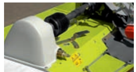
V-belts can be quickly re-tensioned
