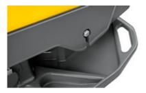
• Tie-down options similar to those of large equipment allow an optimal securing during transport
