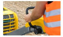
Operator safety: If the operator releases the center pole the vibratory plate continuous vibrating but remains in place (on-the-spot vibration)
