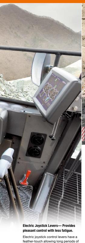
Electric joystick control levers have a feather-touch allowing long periods of effortless operation. Its stroke is much shorter than that of hydraulic control.
