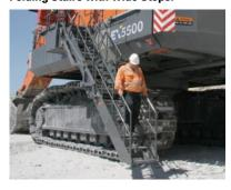
Folding stairs is designed for easy access to the machine for servicing and maintenance.
