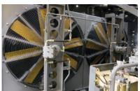
Two oil coolers are used for optimal cooling efficiency. They are positioned far from the engine radiator for even better cooling potential.
