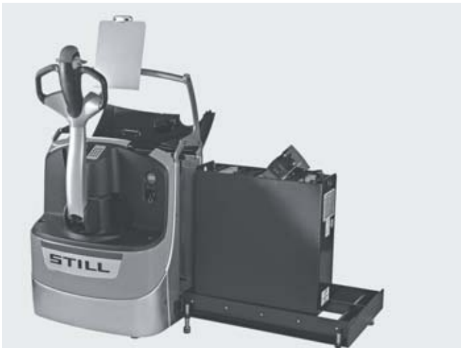
Maximum availability due to lateral battery change
