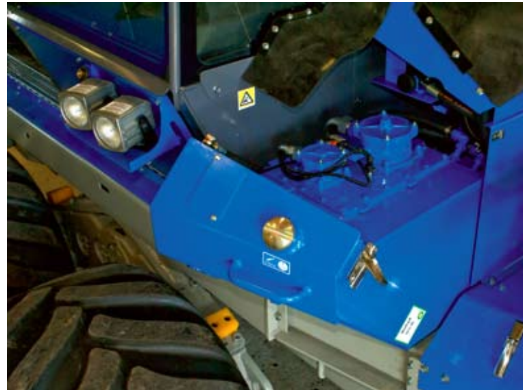
The hydraulic filters can easily be changed when the tank is folded out
