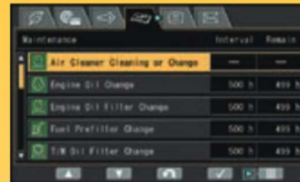
Basic maintenance screen
