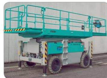
Large working surface with double deck extension (total: 14 sq.m.). Access by lateral double ladder.
