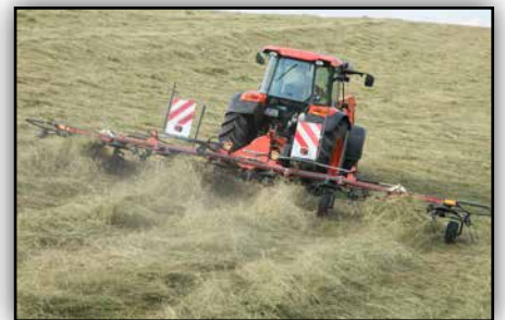
With the optional reduction gearbox it is possible to place night swaths.
