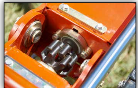
Kubota HexaLink finger clutch permits a 180° folding of the rotors for transport.
