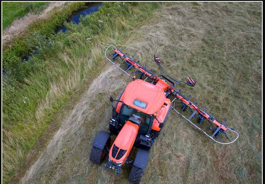
Keep the crop inside the field with border tending, tending the crop away from the border line.
