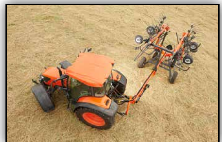
80° turning angle ensures excellent manoeuvrability.
