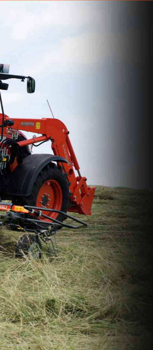
TE8080 folds into a very compact position for transport.
