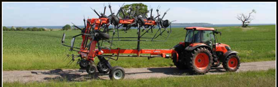
During transport both tedders have a height of 3.35m and a width below 3.00m.
