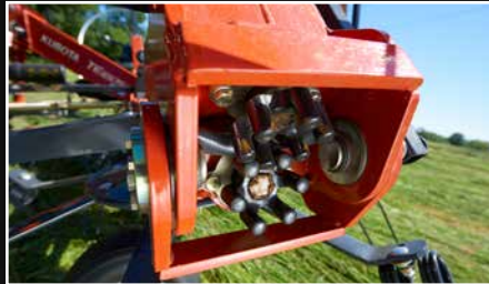
Kubota HexaLink finger clutch permits a 180° folding of the rotors for transport.
