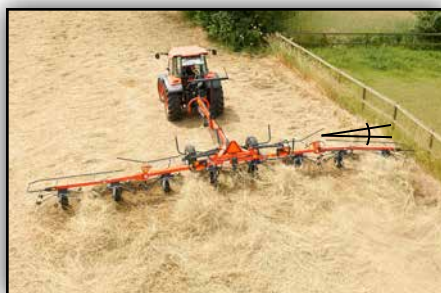
For border tedding the outer rotors are pivoted, to secure evenly inward spreading.
