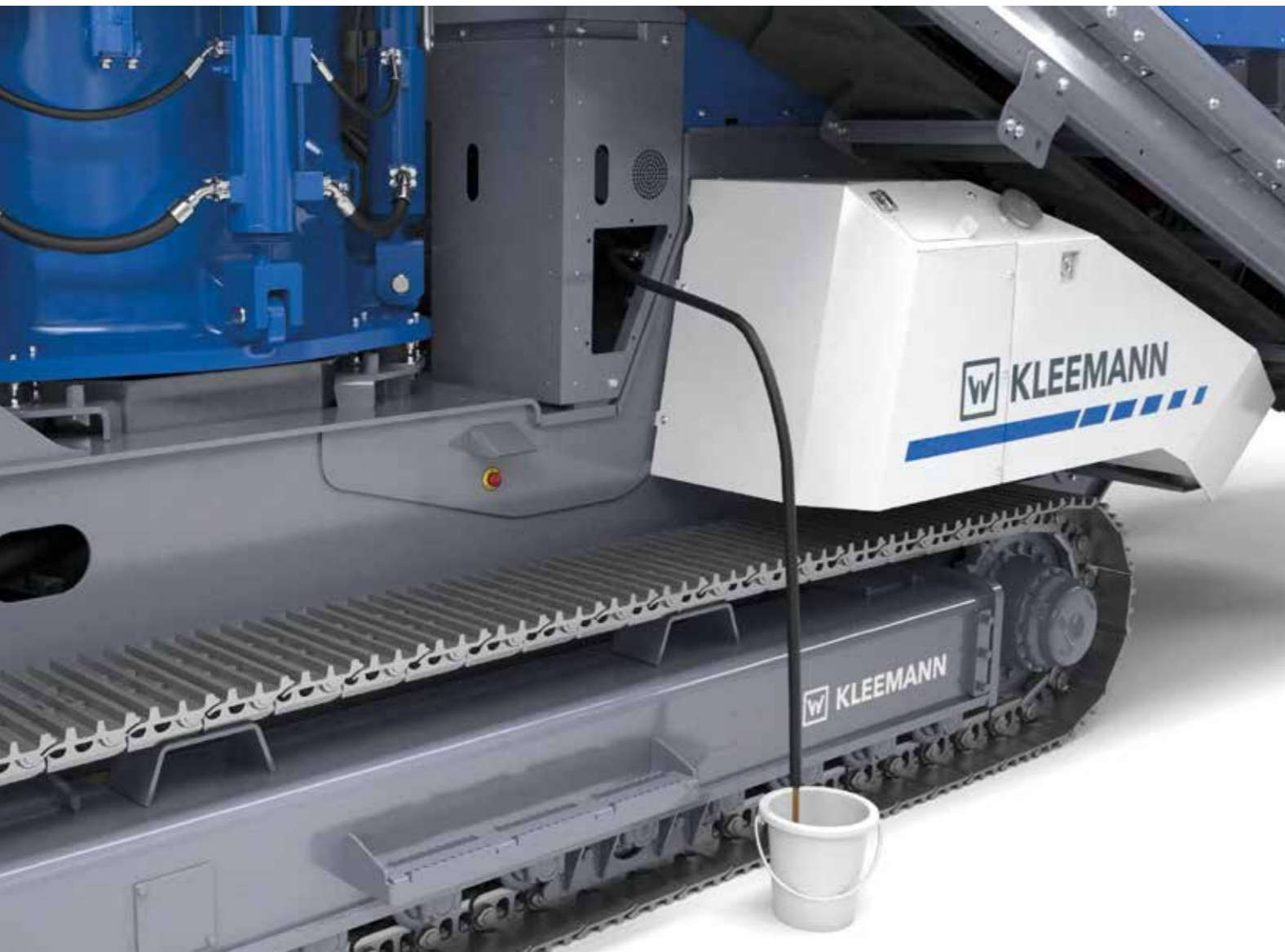
Central drain point
