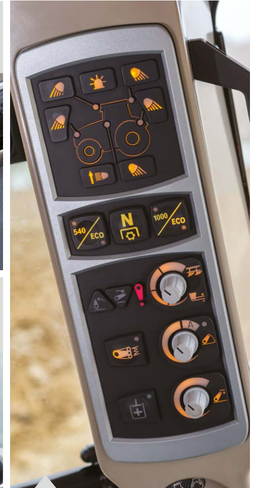
Pillar mounted PTO speed selection controls and linkage controls.
