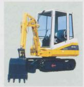
Extra-small min. swing radius and convenient boom offset enable quick dig/load operations in extra tight quarters when close to obstacles. The boom swings 50° to the left and 90° to the right. In addition, the PC10-6 attains a wide working range. Reinforced dozer blade with cutting edge is ideal for refilling and leveling.
