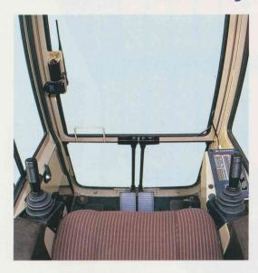
**Human engineered cab** — is both roomy and efficient. The large area of tinted glass allows the operator excellent visibility. Five-way seat with armrests, short stroke wrist-control levers, pull-up front window and travel pedals with levers work together to help your operator maximize production.
