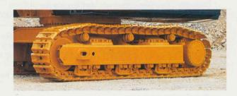
Largest undercarriage components — in its class provides extended life. The same undercarriages are used on Komatsu large bulldozers. In addition, the track motor guards which protect the motors from obstacles are standard equipment.
