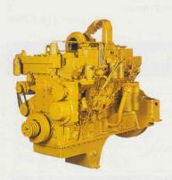
Komatsu SA6D170 diesel engine - assures low fuel consumption. It delivers an ample 405 kW (542 HP) power, making easy work out of heavy-duty digging and loading. And it adopts a directinjection fuel system for greatly improved combustion efficiency. In addition, the lightweight design and reduced friction between moving parts further boost fuel economy. The turbocharger and aftercooler allow the SA6D170 to maintain high performance even on highaltitude jobsite.
