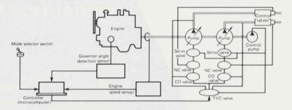
**Electronic Open-center Load Sensing System (EOLSS)** — electronically controls oil flow from the three variable capacity piston pumps so that unnecessary oil flow can be eliminated and fuel consumption significantly reduced. A microcomputer matches oil discharge volume to engine speed (even at high altitudes) so that engine ouput power can be effectively utilized. This also reduces fuel consumption since the engine is not generating unused power.
