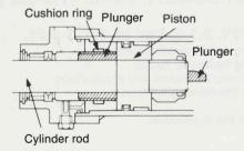
**Cushion mechanism** — in the arm cylinder and head end of boom and bucket cylinders absorbs operating shocks from cylinder extension and retraction, increasing both operating comfort and component life.
