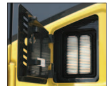
External air conditioner filter
