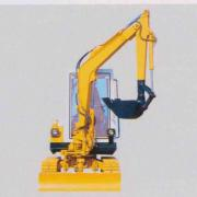
**Convenient boom offset:** The boom itself can be swung  $60^{\circ}$  to left and  $90^{\circ}$  to right side. This means that the PC30-5 can complete quick dig/load operation in extra tight quarters without swinging the upper structure of which the tail end may hit obstacles such as walls, poles, etc.
