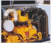
Komatsu-built 3D84 engine provides a tenacious power of 29.6 HP (22.1 kW) at 2700 RPM. Its large piston displacement assures powerful excavation even at partial throttle, without a fear of stalling.
