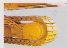
**Two-stage travel speed:** High or low travel speed is selectable depending on traveling conditions. Each travel motor with reduction gears is stored inside the track shoe's width (in-shoe design). As a result, it is protected from external objects.
