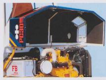
**Full-open machine cover** allows quick access to internal components such as engine, hydraulic equipment, etc. for both quick checking and repairing.
