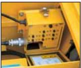
**Circuit breaker** With the circuit breaker, the machine can be easily restarted after repairs.
