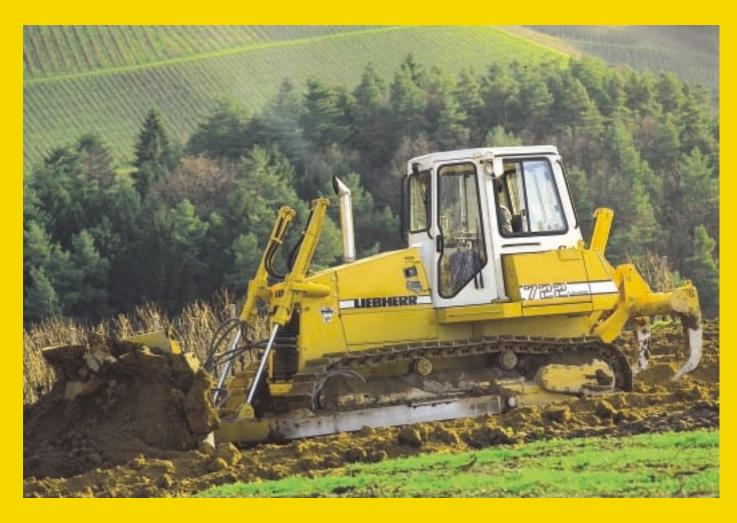
Litronic - A system comprised of intelligent electronics and functional hydraulics - monitors, controls, regulates and coordinates all key systems of the tractor's hydrostatic travel drive.
