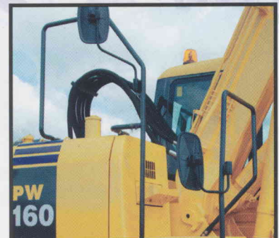
Large handrail for safe access
