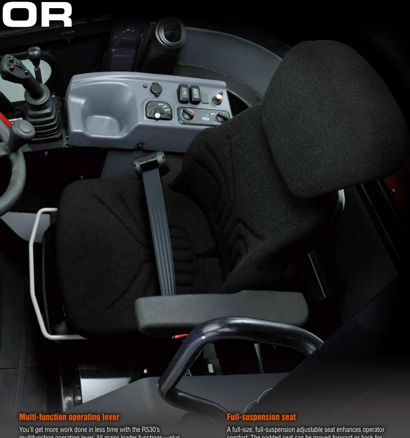
multifunction operating lever. All major loader functions—plus Float, Speed Up/Down, Forward/Reverse, Neutral, and Differential Lock— are on a single lever that is easy to operate with just one hand. The 2-step Speed Up/Down buttons let you quickly change speeds and work at the optimum speed for the task at hand.
