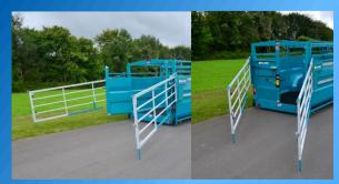
▲ SWIFT side sliding gate mounted on a trolley with spring-loaded parallelogram
