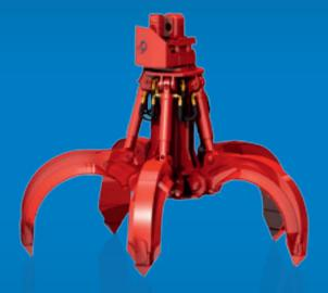
The Rotar Orange Peel Grab has been fitted with a strong rotating headpiece and over-dimensioned slewing ring. The hydraulic motor on the headpiece provides high torque, allowing the orange peel grab to be moved to every possible position.
