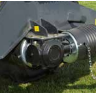
540/1000rpm turnable gearbox as standard.
