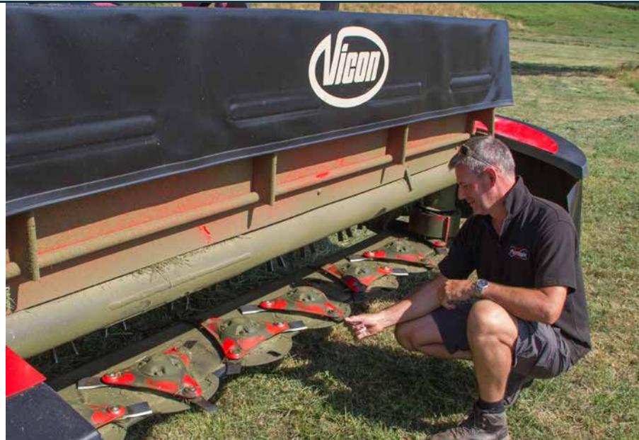
Front cover is opened into a vertical position for easy access.
