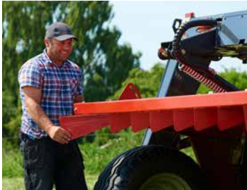
Dismount the two deflector doors and you are ready to mow.
