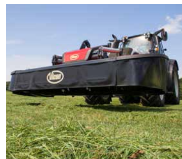
Generous ground clearance for headland turns of 420mm to pass large swaths without damaging them.
