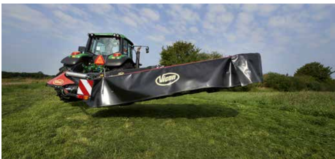
Lifting on headlands via hydraulic cylinder – ample ground clearance.
