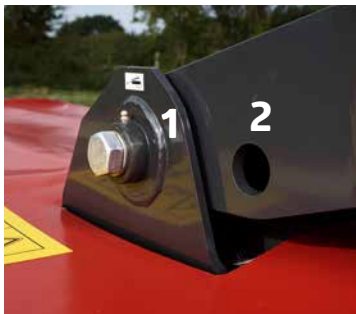
Two mounting options for optimal overlap with a front mounted machine.
