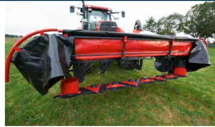
Easy access to the cutterbar with foldable front and side guards.
