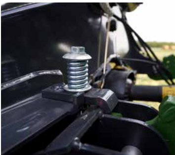
When encountering an obstacle the NonStop BreakAway system protects the cutterbar by swinging it back and up.
