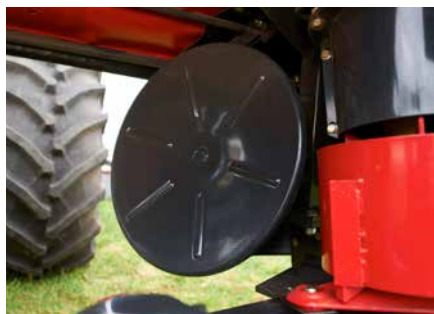
The machine is standard equipped with two swath discs, allowing a swath width of 2.20-2.40m.
