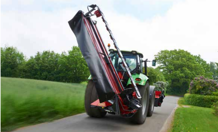
Up to 125° vertical transport position for excellent weight distribution.
