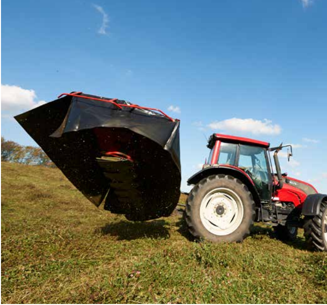
Lifting on headlands via a hydraulic cylinder.
