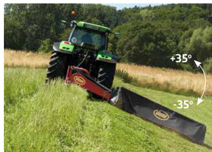
The design allows mowing at extreme angles.
