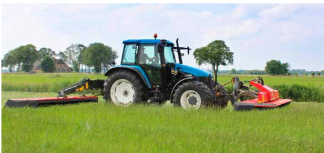
Centre mounted suspension for even weight distribution and fast adaptation to ground contours.
