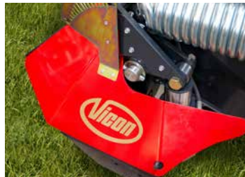
Hydraulic on-the-go setting of ground pressure (optional).
