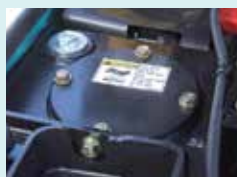
Hydraulic oil tank
