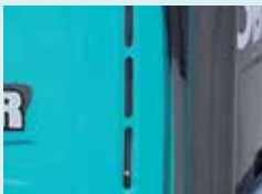
Fuel tank gauge
