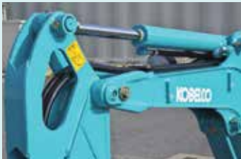
Bucket cylinder hoses sited within the arm
