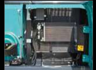
Left side (radiator and cooling system elements)
