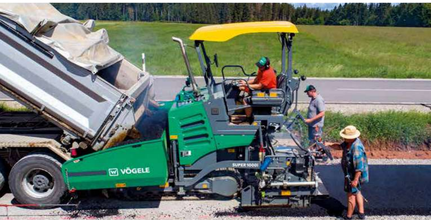
The power unit of the SUPER 1000i with diesel oxidation catalyst (DOC) and diesel particulate filter (DPF) for exhaust gas after-treatment complies with the strict requirements of European exhaust emissions standard Stage V and US EPA Tier 4f.
