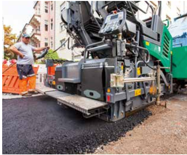
AB 340 V built up with 25cm bolt-on extensions
