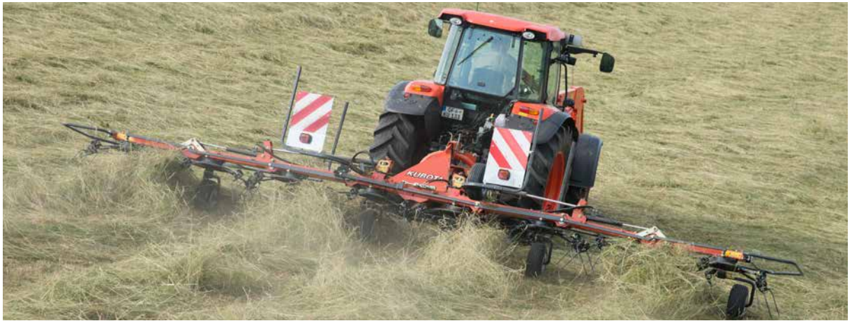
With the optional reduction gearbox it is possible to place tight swaths.
