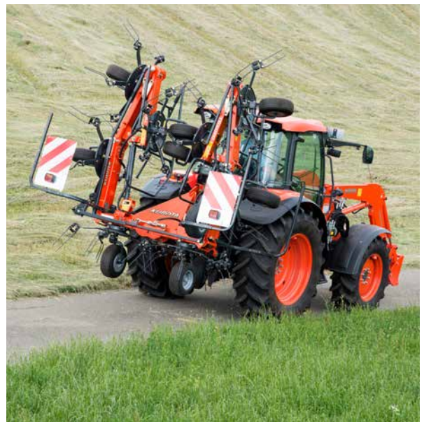
TE8080 folds into a very compact position for transport.
