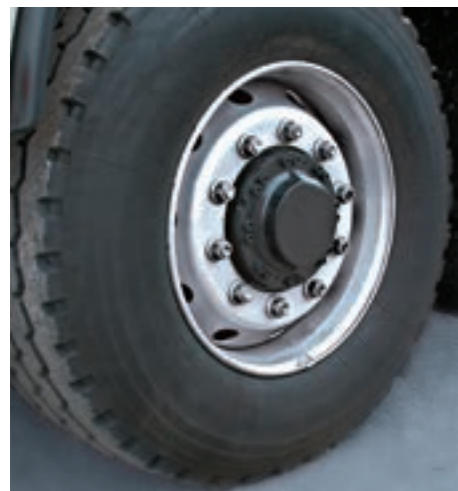
Front axle with hydrostatic wheel hub motors
