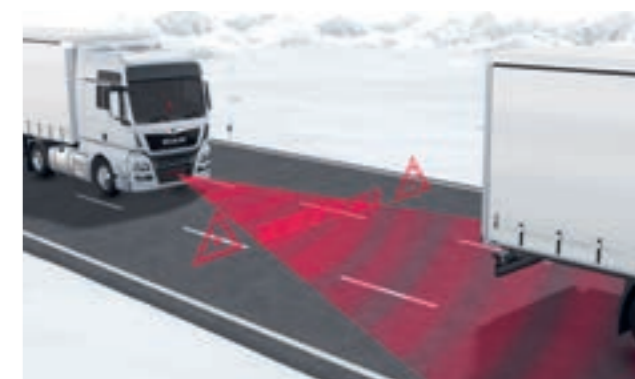
Functional principle EBA: advanced traffic monitoring by using two independent sensor systems (radar and video)
