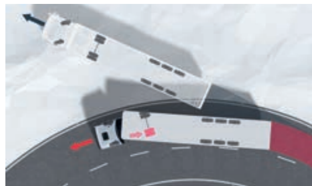
ESP compensatory braking when vehicle is understeered
