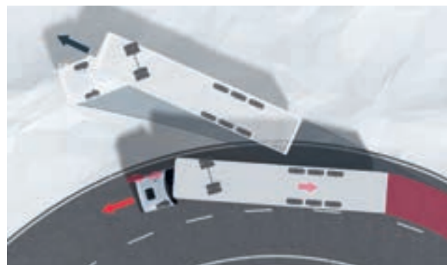
ESP compensatory braking when vehicle is oversteered
