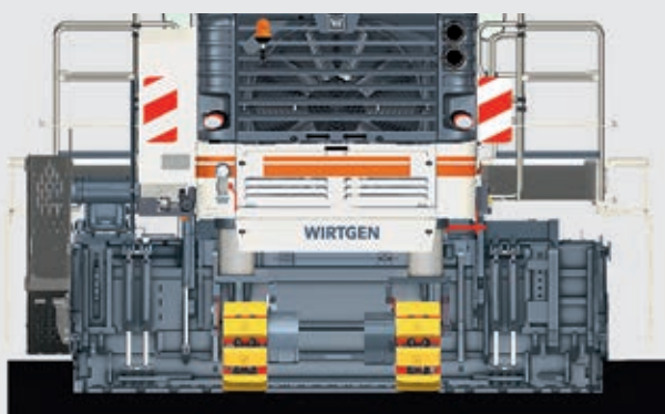
W 250i with 3.8-m drum assembly
