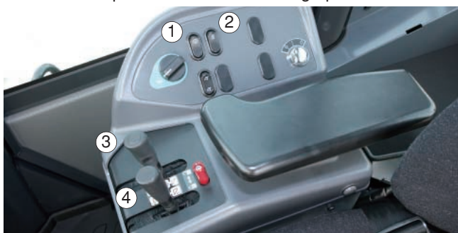
1:Cut-off ON/OFF switch 2:Cut off adjustment switch 3:Boom control 4:Bucket control
