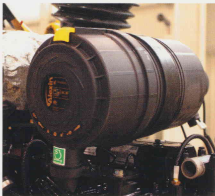
Improved Air Filtration Donaldson Filter
