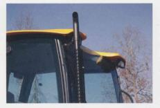
**Corner Exhaust/Front Roof Cut-out**
