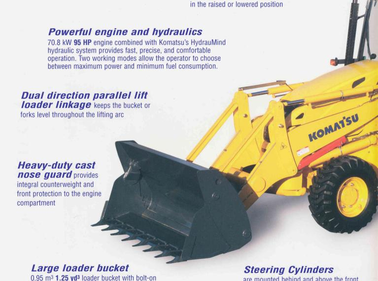
NET HORSEPOWER 70.8 kW 95 HP @ 2200 rpm
