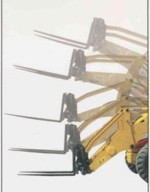
Mechanical linkage design keeps the load level from bottom to top (max 11° tilt back).
