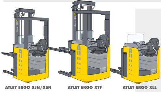
The Atlet ERGO XLL is intended for convenient and frequent movement of materials and pallet goods. It can be driven easily onto a lorry platform.
