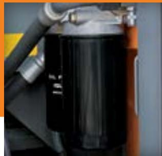
■ Easily installed spin-on main fuel filters help prevent contamination when servicing. Two additional water separators help extend fuel filter life.
